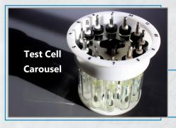
The BLB Test Cell Carousel accommodates twelve (12) samples, allows convenient alignment of each cell to the appropriate test position, and holds both  $\mathsf{SimAir}^{\mathsf{T}}$  and  $\mathsf{DIN}$  glassware.
